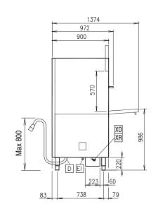
Drain ΕI Electrical inlet (power) EO **Electrical Outlet** HWI Hot water inlet
